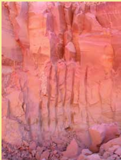
A section of the Hayricks boulder opal mine, located in central to northern Queensland, Australia. Scratches on the face of the mine were made by a large diesel backhoe used to scoop material daily.
